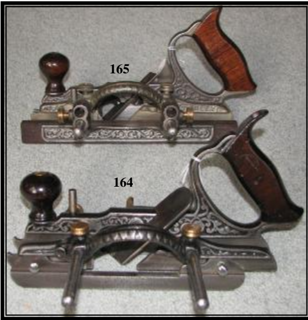
164 Stanley No 46 adjustable Dado Plane complete with fence & depth gauge C. 1873 F 300-500 Trouts Patent Adjustable Dado Plane Type 2 complete with fence & depth gauge C.1873 F 900-1000
